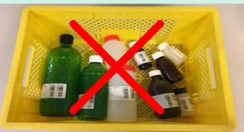
Bottles firmly placed in crate, do not protrude above edge
